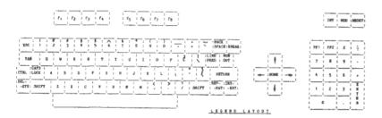
There are 10 user programmable function keys provided. Eight of these are fully supported by high level languages and CODOS. Their "TITLES" are displayed on the 25th line on the CRT (bottom line) enclosed in 8 rectangular boxes. Their functions can change dynamically under software control, reducing the need to "remember" what functions can be done in which "modes".
